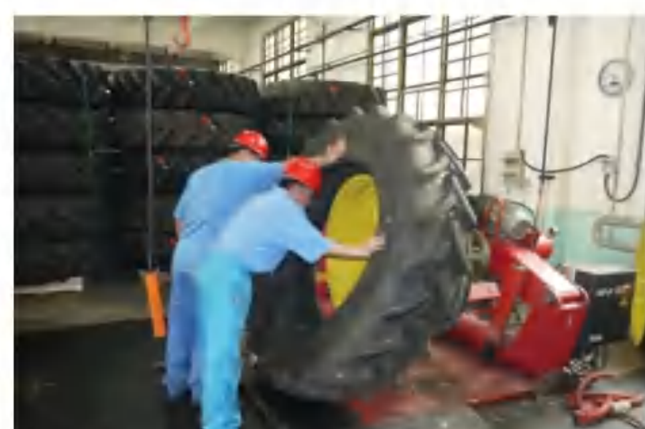
轮胎轮辋装配 Tire and wheel rim assembly
