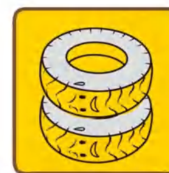
短期（30天）存放， 可以平放地面。 Short term (30 days) storage, can be placed flat on the ground
