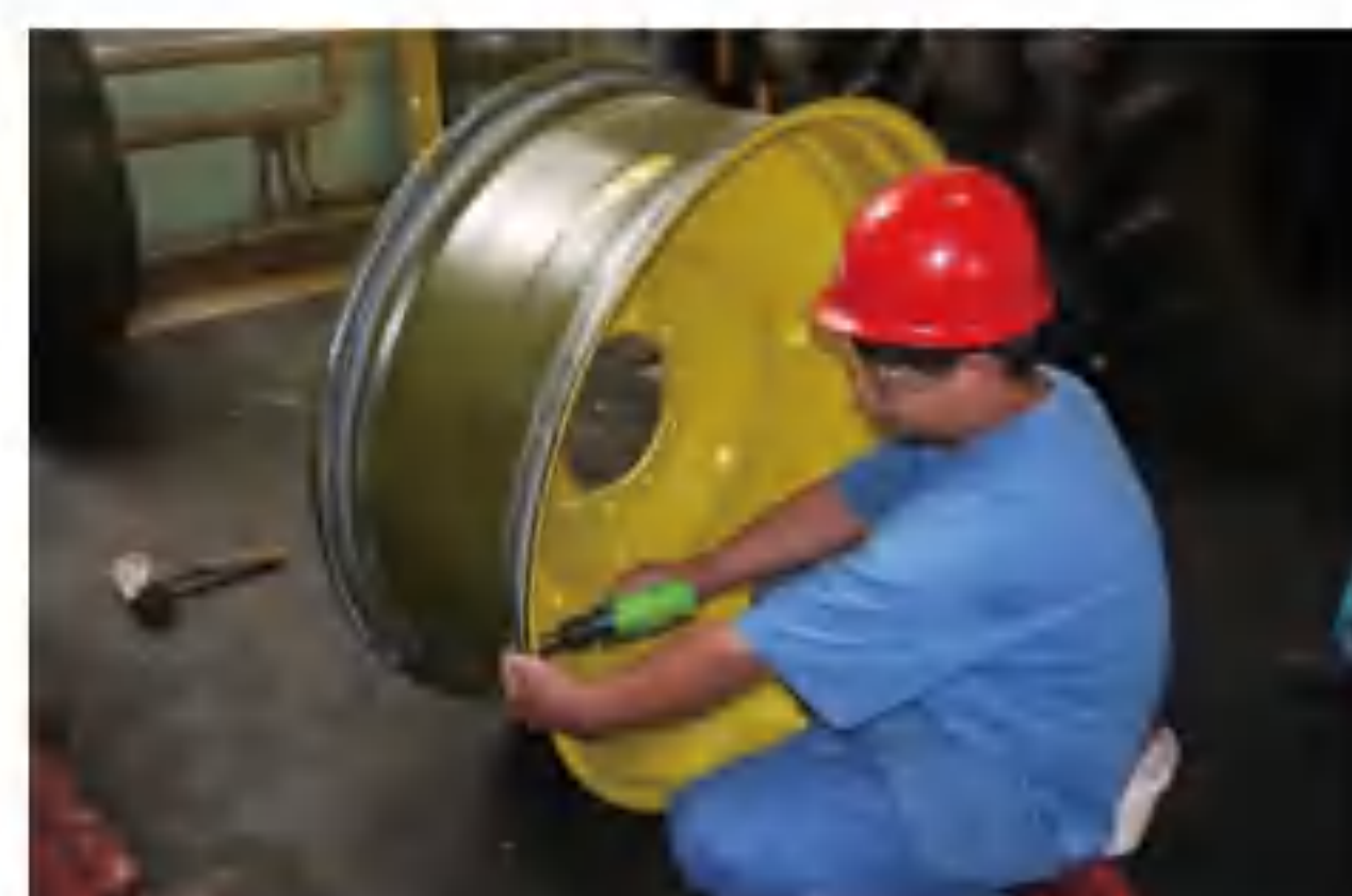
安装气门嘴 Install the valve
