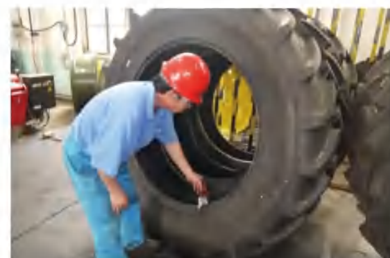
轮胎趾口涂抹润滑脂 Apply lubricating grease to the toe of the tire
