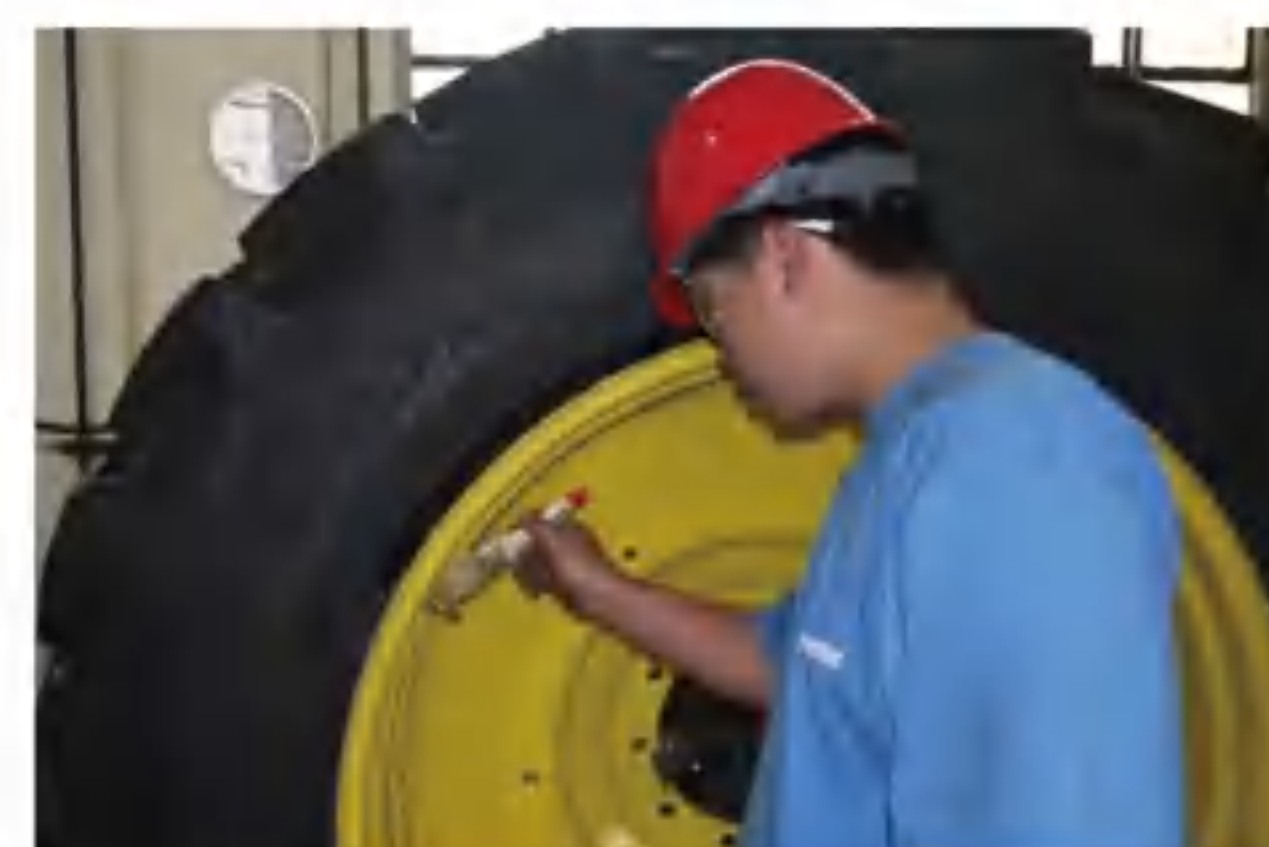
检查胎圈密封 Check the sealing of the tire bead
