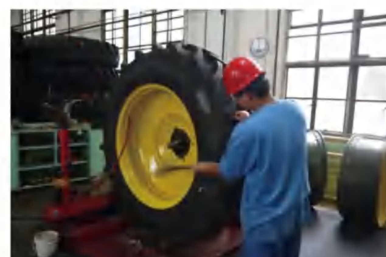
检查轮胎趾口与轮辋结合 Check the connection between the tire toe and the wheel rim
