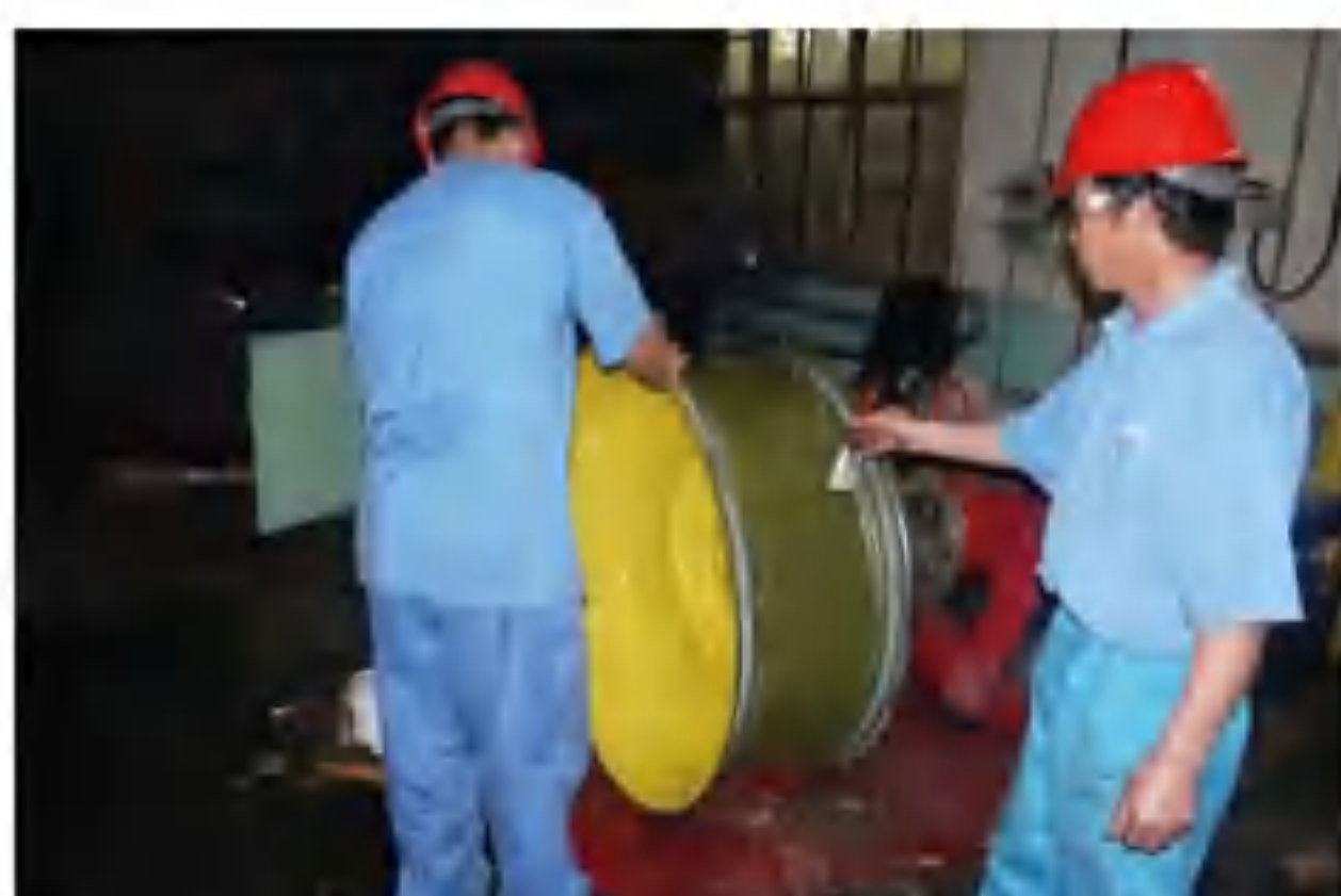
轮辋涂抹润滑脂 Apply lubricating grease to the wheel rim
